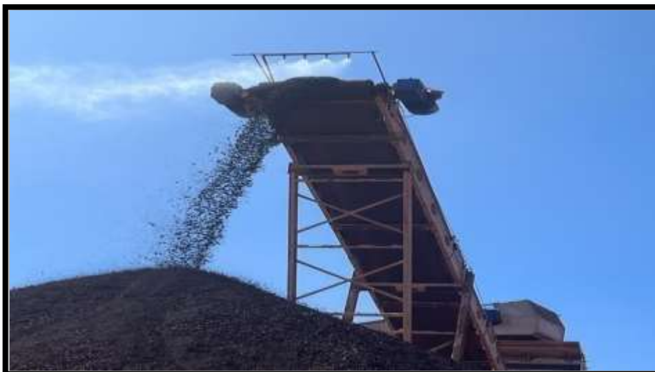
Dry Fog System in Mineral Handling Plants
